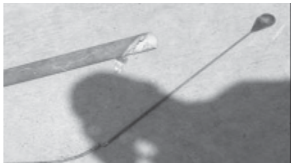
Photo 2. Support Mast melted through on one side
